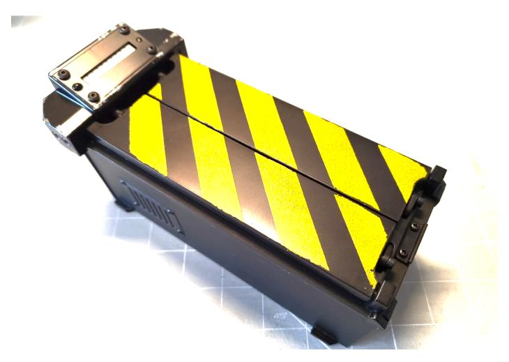
The inner removable section of the Haslab Ghost Trap (which we will refer to as the 'Cartridge') is the assembly that consists of the inner chamber, doors, bargraph, indicator light and front control dials. Inside the cartridge is where you will find Hasbro's main circuit board that controls the door mechanism, chamber LEDs, bargraph LEDs and takes input from the front dial switches and the PKE IR sensor.
