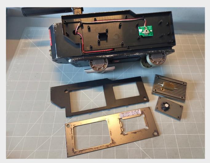
You can now pull off the two small plates with the resistor and rotary knob, the large metal side plate and the black plastic insert.
