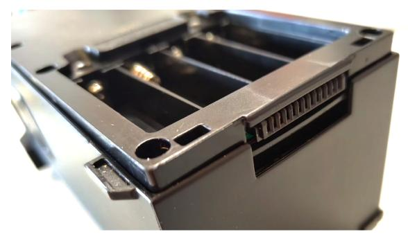
We can now gain access to the inside of the cartridge. Start by gently pushing up at the connector end until the bottom section releases as shown above.
