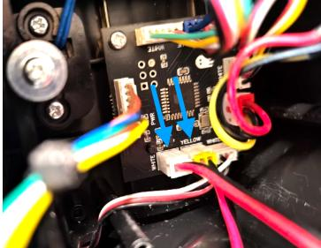
Bring back the base plate and connect the two remaining cables as shown above. If you have installed a new speaker and replaced the cable, this need to be attached to the connector labeled 'YELLOW'.
