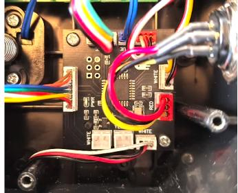
Position the square board behind the loose wires inside the chassis and connect each of the six cables to their respective connector. These are clearly printed on the board itself (small 5-pin WHITE, small 4-pin WHITE, small 3-pin WHITE, large 3-pin RED, small 3-pin RED and small 2-pin BLUE).
