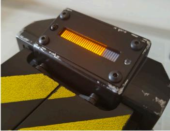
Now place the glossy window film over the top of the lens - you may want to give this a wipe with a clean soft cloth to remove any dust and fingerprints. Finally, reattach the face plate using the four button head screws we removed earlier. Et voilà! You now have a beautiful 30-segment bargraph display!
