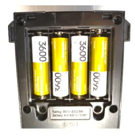
Lithium-ion batteries, on the other hand, are able to maintain a steady voltage throughout the duration of their lifetime, so your Trap will continue to function correctly until the batteries are fully drained and ready to be replaced or recharged.
