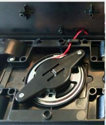
You will now need to desolder the cable attached to the old speaker and attach it to the new one. Solder the red wire to '+' and the black wire to '-'. You can now place the new speaker into the circular cutout in the chassis base plate. Note that you may need to trim a little bit of the plastic away from inside this cutout so that the speaker sits flat.
