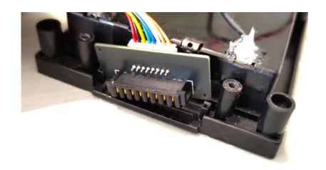
Connect the 8-wire cable to the connector board. Note that there are two similar looking connector boards included with your kit, so make sure you are using the one labelled 'CARTRIDGE CONNECTOR'. Now insert the board into the slots on the bottom plate with the black pin connector facing outwards.
