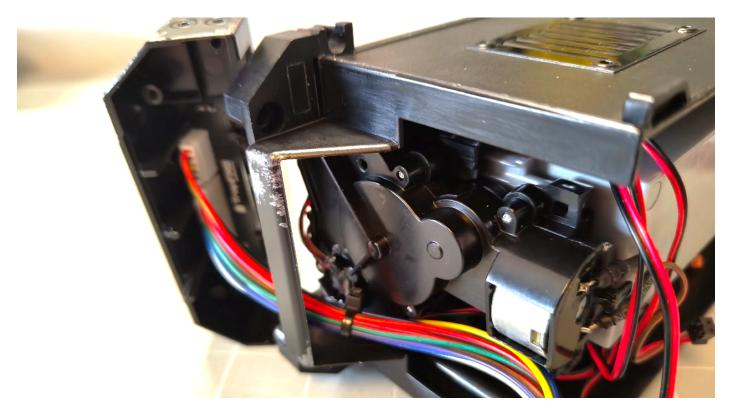
Thread the cables through the front hole in the cartridge and reattach the bargraph section by replacing the four screws and caps we removed earlier.
