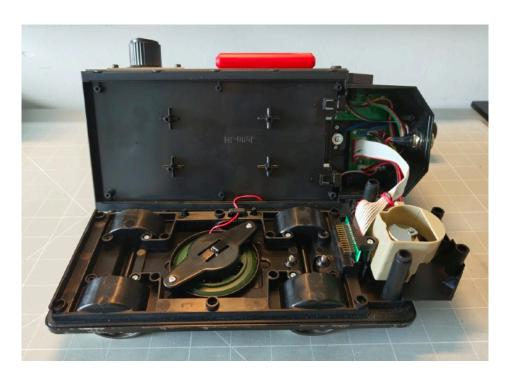
Sit the trap on its side with the red/silver rods facing upwards, and carefully pull the base plate away from the chassis and place it down on your table. Be aware that there are two cables attached here, so do not pull the base away too sharply as the wires can easily be broken.
