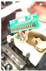
Turn your attention to the connector board which is recognisable by its 13 gold pins. As with the cartridge, this is secured in place by a plastic holder. Remove the two screws **circled** above take off the holder. Note that these screws are longer than the others, so keep these aside separately with the holder so they don't get mixed up. You can now lift out the connector board.
