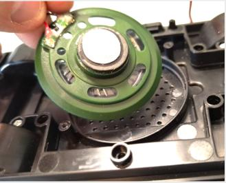
Remove the two screws **circled** above to release the plastic speaker holder. The preinstalled green speaker can then be lifted out.
