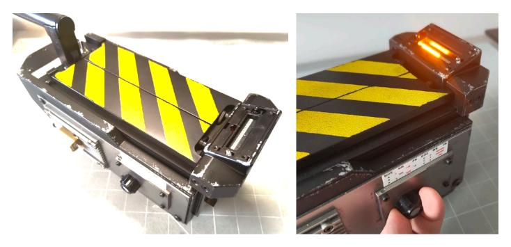
Great! That's all the new electronics installed, but we still need to get that bargraph looking good. Slide the cartridge into the chassis until it clicks into place and turn on the power by rotating the SYNC dial clockwise on the front of the trap. Now rotate the side knob in both directions - you should see the bargraph LEDs filling up and emptying as you do so.
