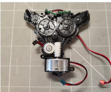
Lay the mechanism assembly flat on your bench once again and slowly remove the top plate. This will reveal the mechanism itself that includes eight plastic gears along with the motor that we will be replacing.
