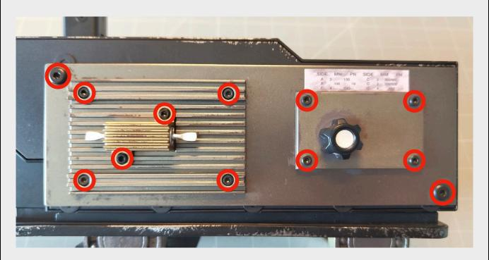
In order to swap out the speaker, we must first remove the chassis side plate that includes the resistor and rotary knob. Use allen keys to remove the twelve black bolts as **indicated** above.
