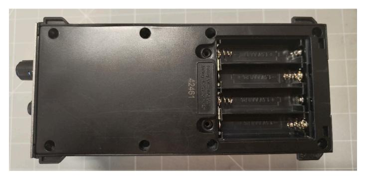
The bottom plate should fit back into place easily and sit flush with the bottom edges of the cartridge. If there is any resistance, you may be pinching a wire. In this case, open up the cartridge again and check the position of your wires until the bottom plate sits correctly.
